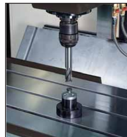
Automatic Tool Length Measuring Device
