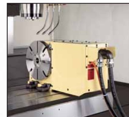
Rotary Table With 4 th Axis Control
