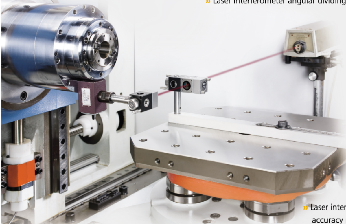
» Laser interferometer angular dividing accuracy measurement.
