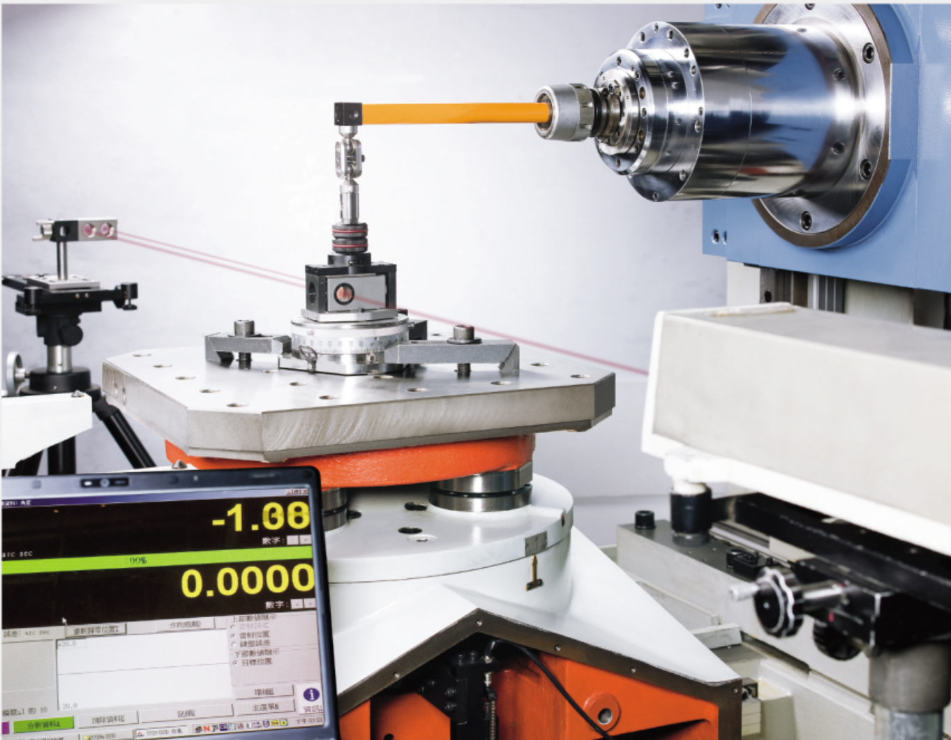
» Laser interferometer angular dividing accuracy measurement.
